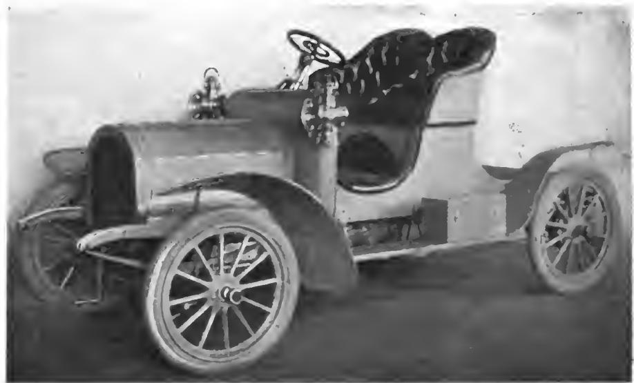
PAGE 10-HORSEPOWER AIR-COOLED RUNABOUT WITH INDIVIDUAL CLUTCH TRANSMISSION.
